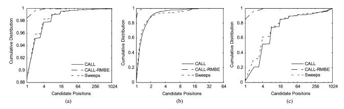
Fig. 6. Cumulative distribution of the possibility. (a) Number of candidate positions for each single node. (b) Average number of candidate positions in each network instance. (c) Maximum number of candidate positions in each network instance.
